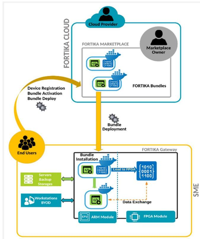
**Figure 2. Deployment of bundle to FORTIKA GW**
